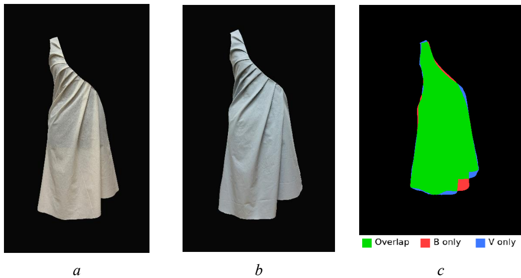
Figure 5.7 — Silhouette Comparison of the Target Dress B and Validation Dress V: a — target dress B; b — validation dress V; c — silhouette-overlay result after centroid alignment
