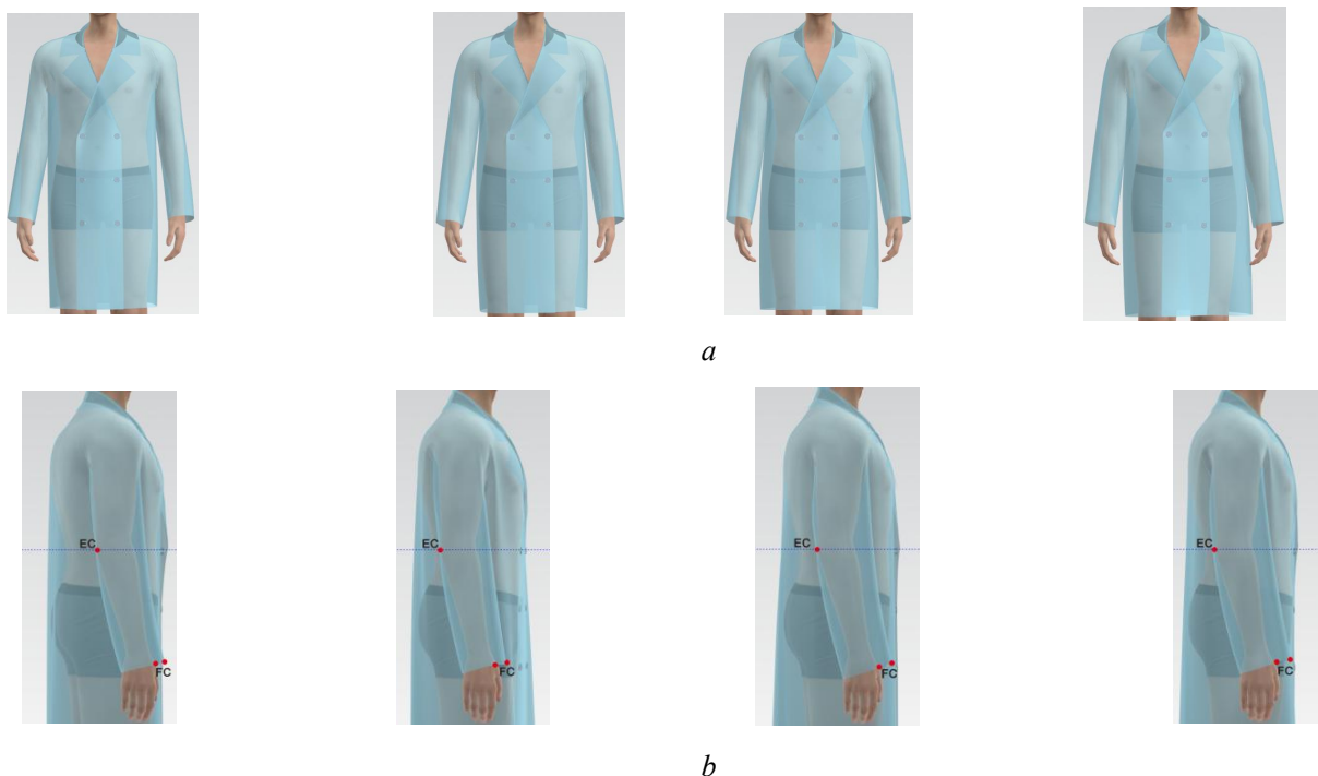
Figure 2.13 - Choosing second criteria EC for air gap between elbow point and sleeve for raglan coat with different E(CG) = 12, 16, 20, 24 cm: a - front silhouette of different E(CG) , b - profile silhouette of different E(CG) )
