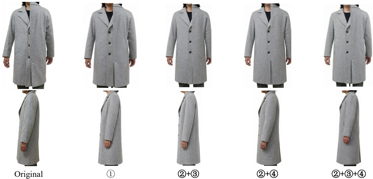
Figure 4.14 Original defective sample and iterative refinement results generated based on the defect diagnosis results in Table 4.8: Original; ① center-front regularization; ②+③ sleeve centerline refinement and fold reduction; ②+④ sleeve-line refinement and cuff–arm spatial adjustment; ②+③+④ integrated refinement.
