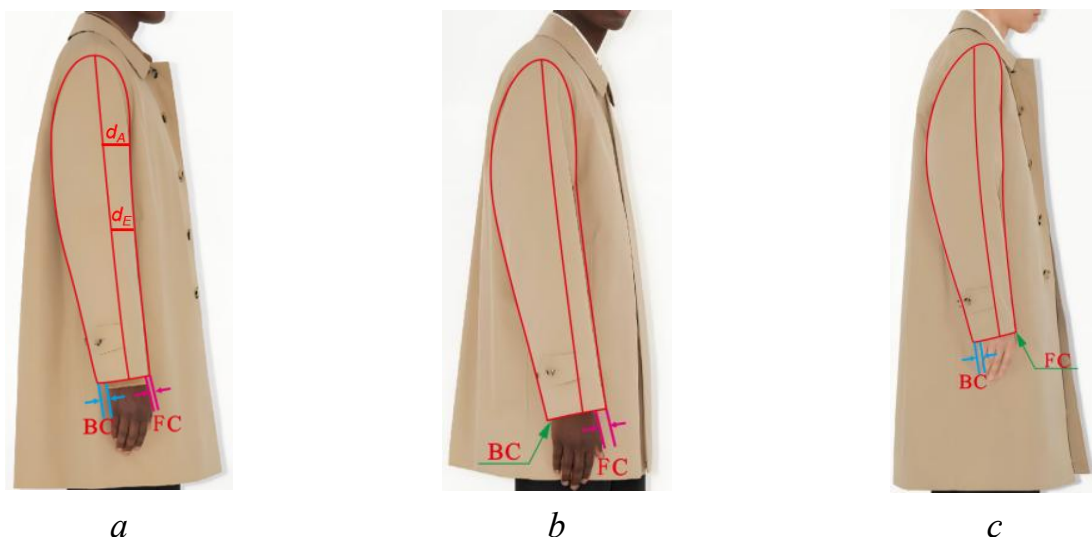
Figure 2.10 - The scheme of air gaps measuring and possible position of cuff and hands: a - arm in the neutral position, b - BC=0, c - FC=0
