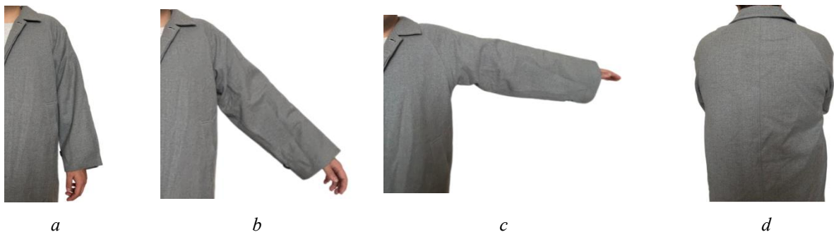
Figure 1.19- Dynamic evaluation: a - Lowering; b -side raise, c -Horizontal raise; d -Cross arms over chest
