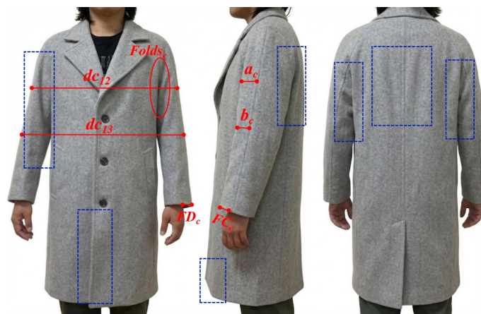
Figure 5.7 - Photo-based analysis of the target raglan coat: blue dotted lines indicate localized shape defects; red solid lines indicate the measured shape parameters.
