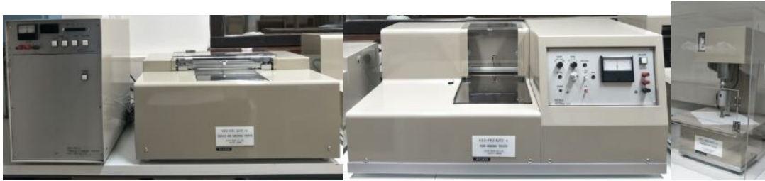
Figure 3.1 - KES-FB1, FB2, FB3 instruments
