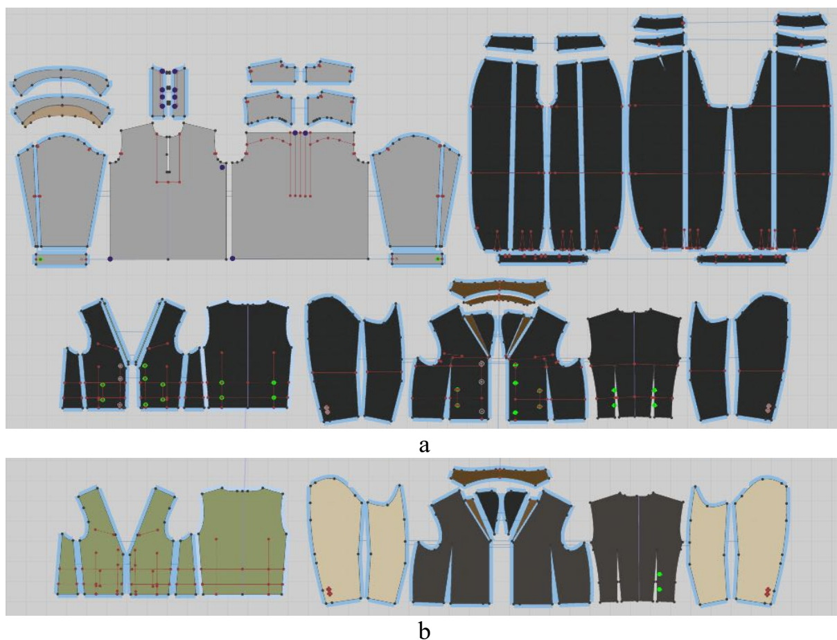
Figure 5.6 – Pattern block of four garments of the uniform: a – shell of shirt, trousers, waistcoat and jacket; b – lining of waistcoat and jacket
