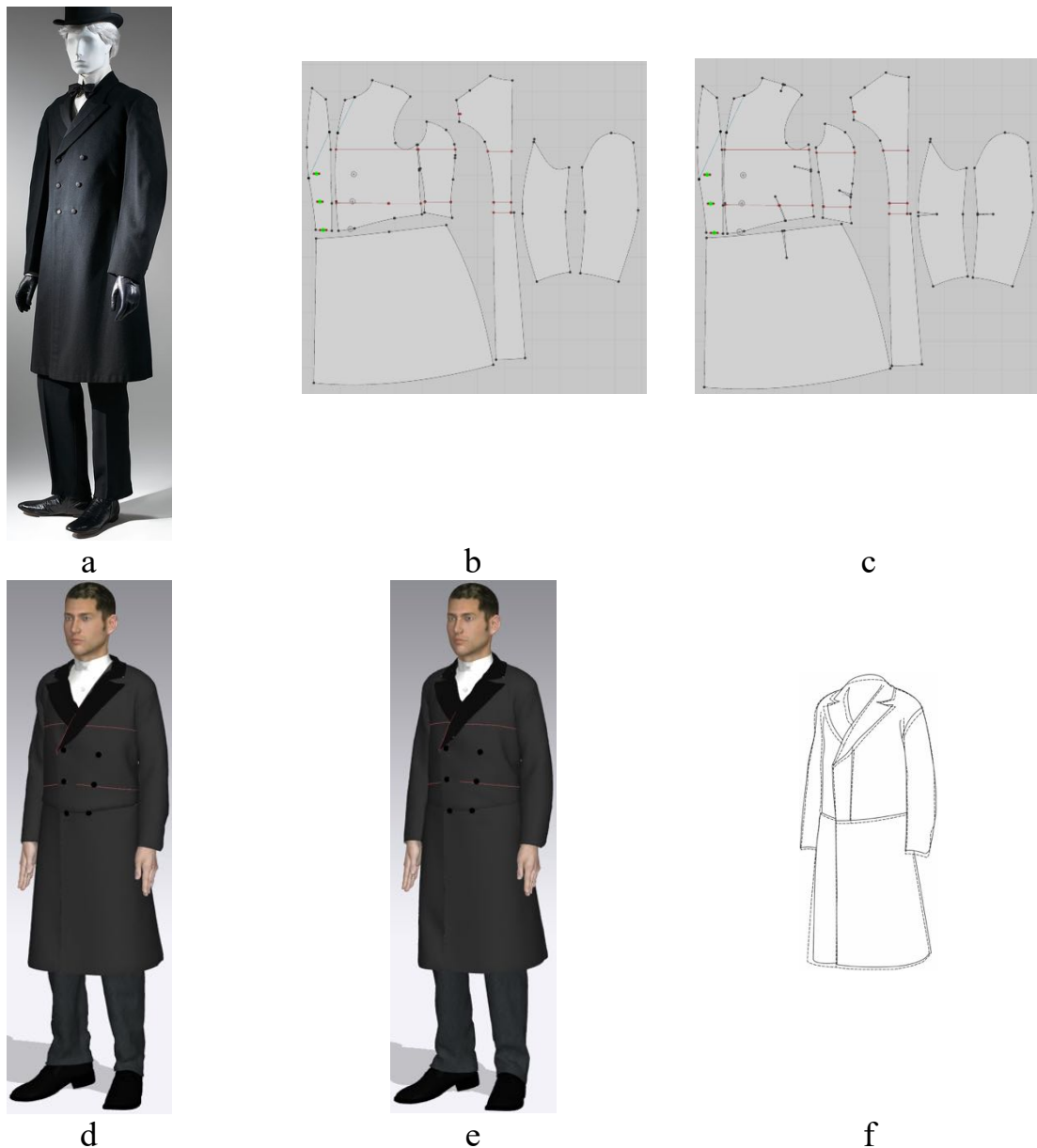
Figure 3.22 – Get DT of men's coat: a – original image [148]; b – original pattern; c – modified pattern for virtual try-on; d – DT of original coat without adjusting the suture lines; e – DT of coat, generated according to the modified pattern; f – combined the contours of DT
