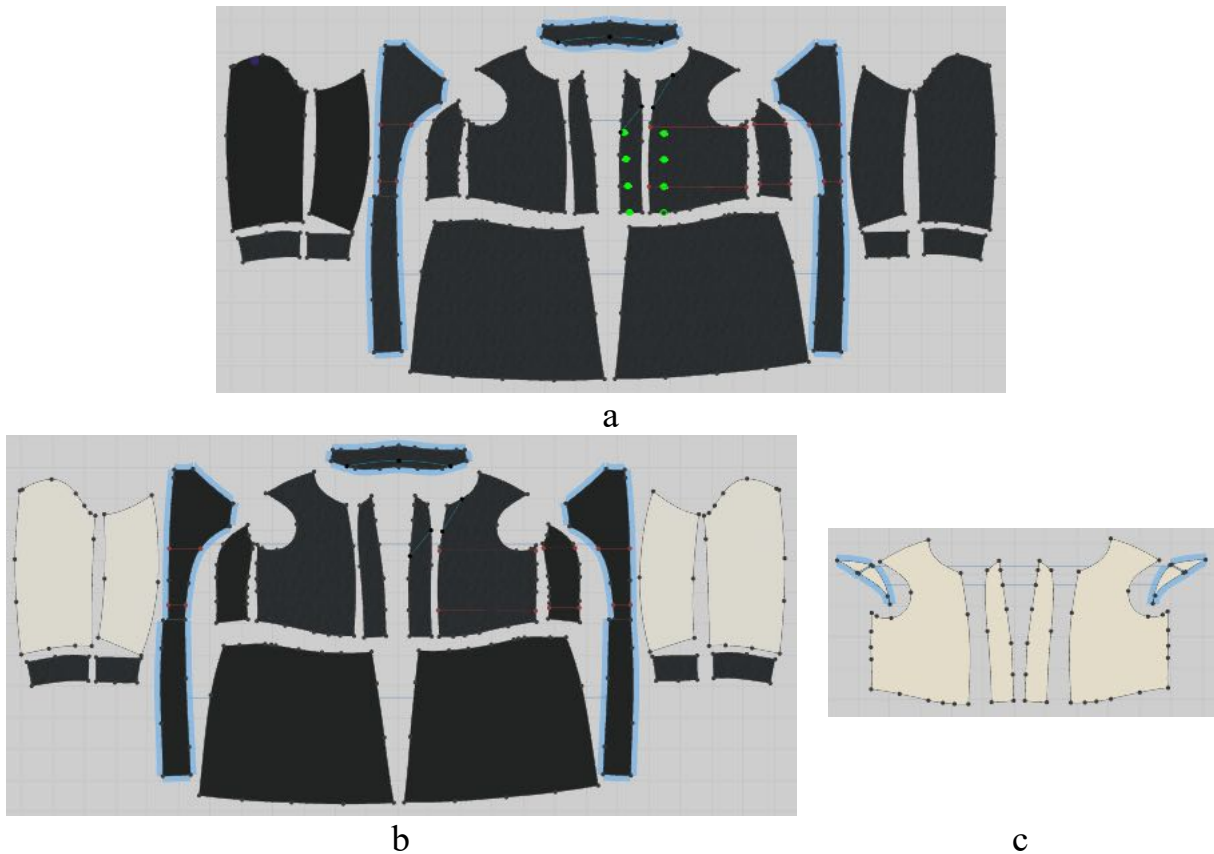
Figure 3.3 – Screenshot of the complete set of pattern of the coat in CAD: a - details of the top fabric; b - details of the lining; c - paddings
