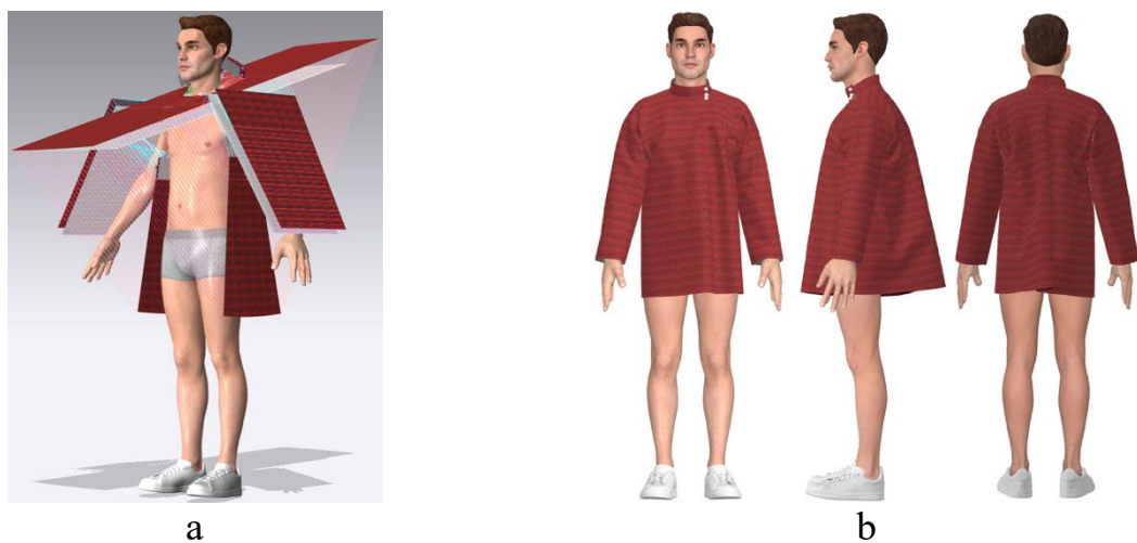
Figure 5.9 – DT of Russian folk shirt : a – 3D arrangement; b – three views of virtual shirt
