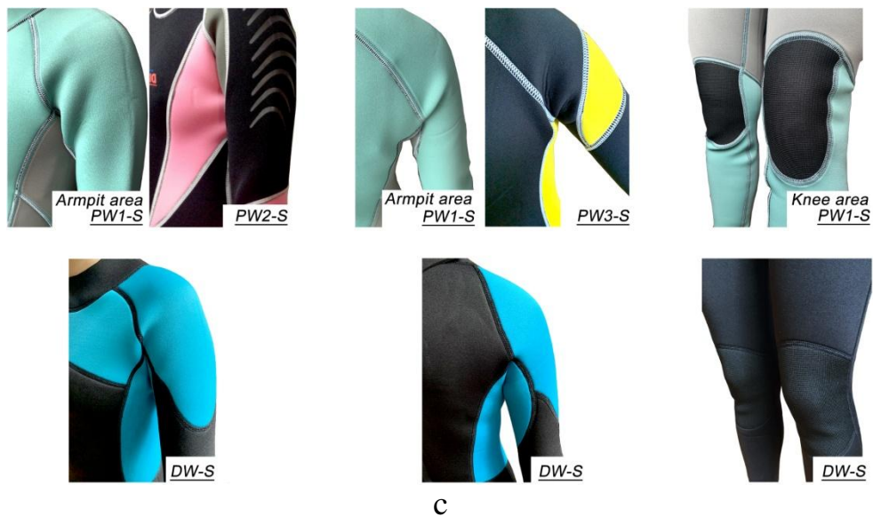
Figure 5.17 – The appearance of the existing PW factory-made wetsuits (a – in the Y1 body; b – in the A1 and B1 bodies) and the appearance of problem areas on the existing PW and the developed DW wetsuit (c)
