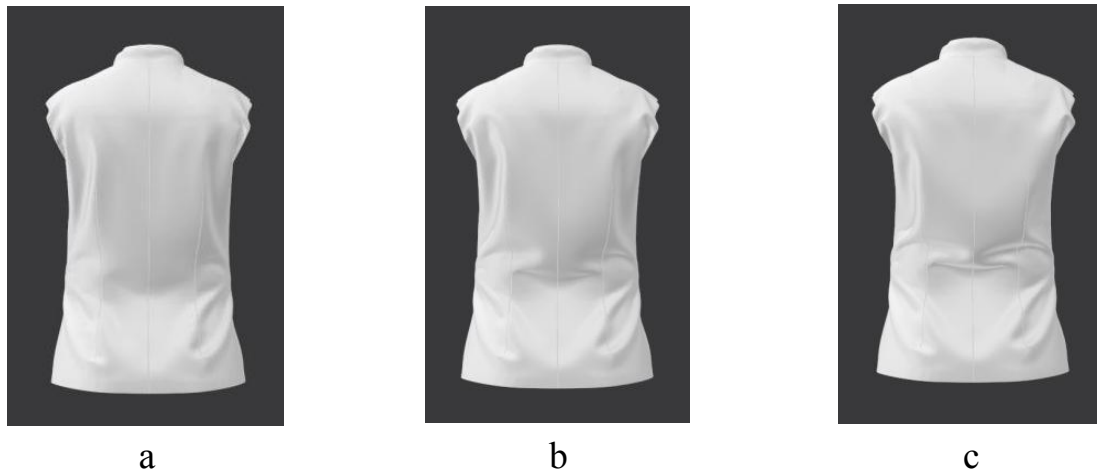
Figure 4.3 - Women blouses with folds causing by ease allowance to back length ( E_{BL} ), cm: a - 3, b - 4, c - 5
